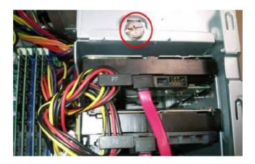
4.2 Disconnect the SATA HDD cable and HDD power-cable from the rear of HDD and MB
